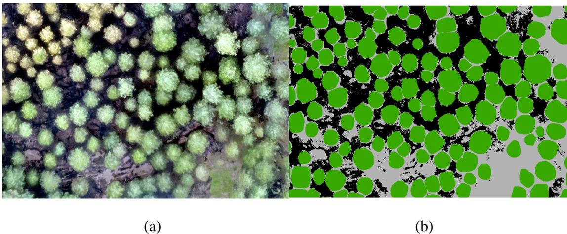
Figure 6 - Part (a) is an orthomosaic of Hoodoo that was created using drone imagery. Part (b) is the Hoodoo image classified into tree pixels (green), burn pixels (black), and surface pixels (grey)
