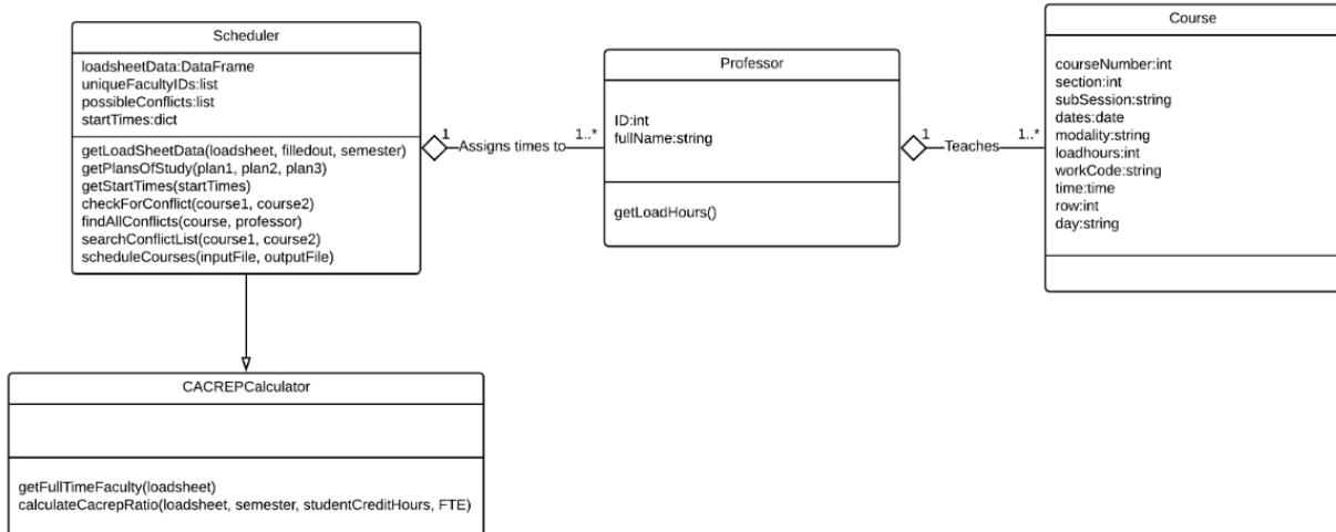
**Figure 3 - Class Diagram**
