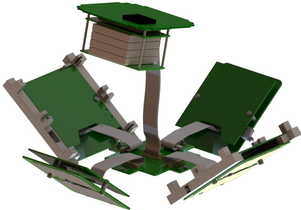
Figure 2: MakerSat CAD Exploded View
