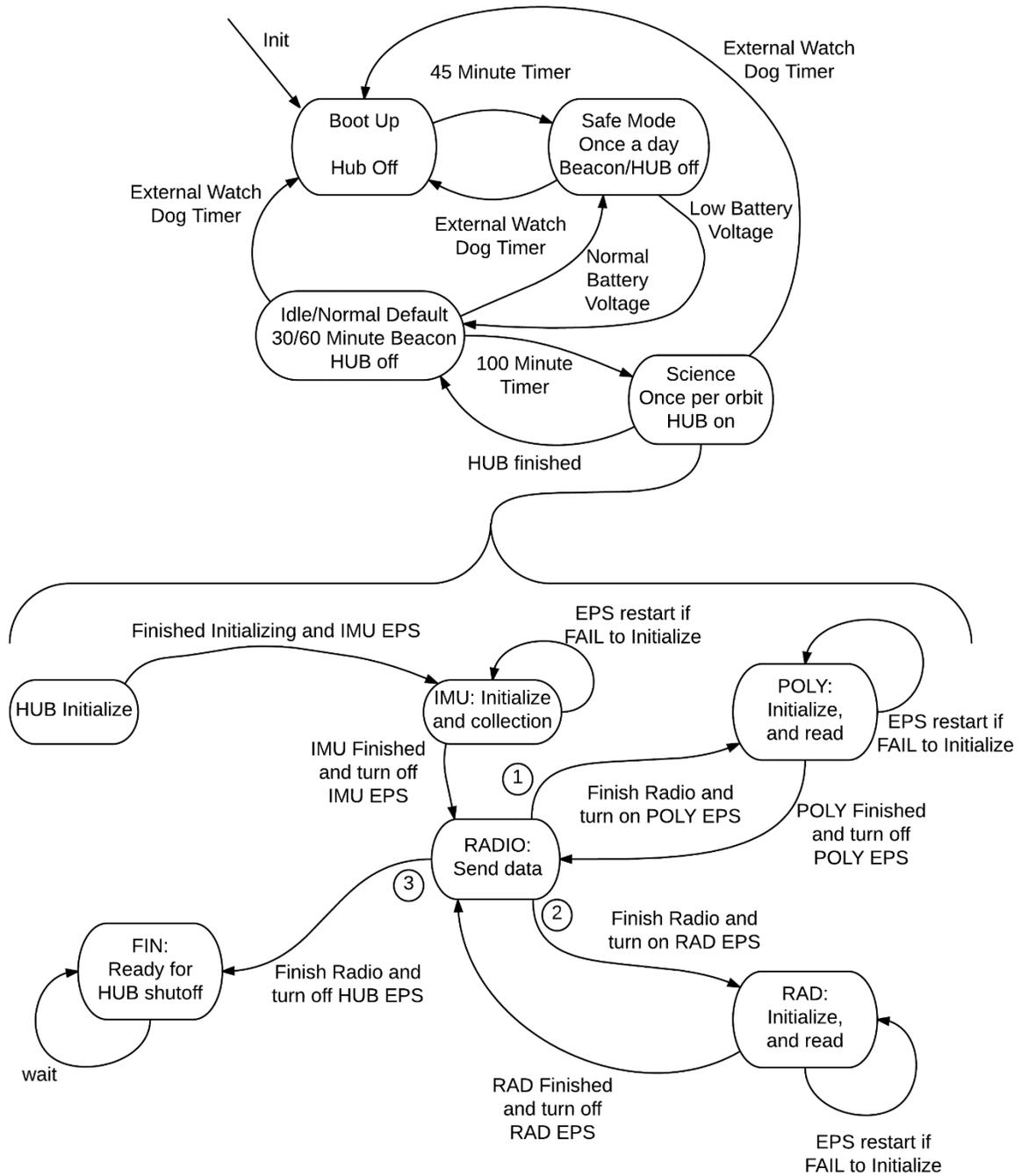
Figure 3: Finite State Machine Diagram
